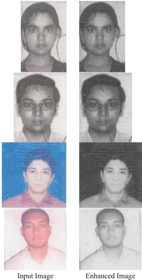
Fig. 3. Examples of enhanced scanned and digital face images obtained using the proposed DWT fusion algorithm.
