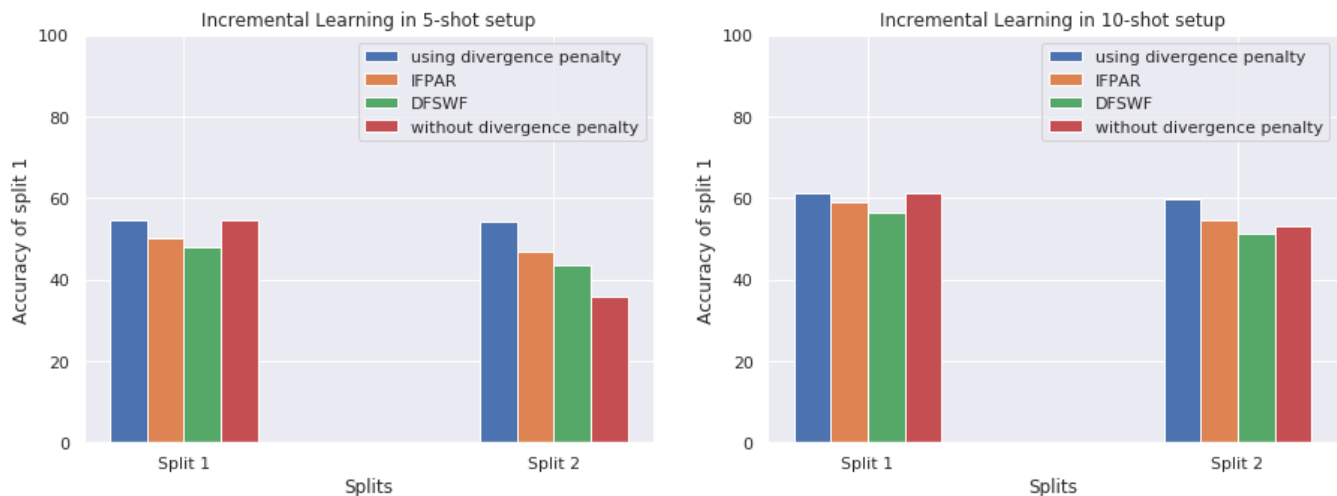
Figure 2: Demonstration of effect of our proposed divergence penalty on the accuracy of the first split as new split is added in i) 5-shot incremental learning setup and ii) 10-shot incremental learning setup. In the 5-shot setup the divergence penalty improves the performance on the first split by 18% and 6.5% in the 10-shot setup compared to when divergence penalty is not used. Comparison with IFPAR (Xiang et al. 2019) and DFSWF (Gidaris and Komodakis 2018) is also shown.
