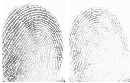
Fig. 2. Difference in image quality can cause reduced performance: 35 years old housewife in rural settings (second image with heena/mehandi applied on the finger).
