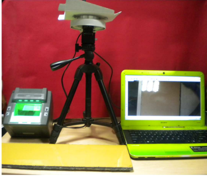
Figure 3. Camera setup for IIITD SLF database capture.
