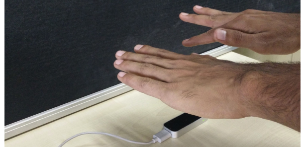
Figure 1: Acquisition of Leap password: the subject is performing fingertap gesture.
